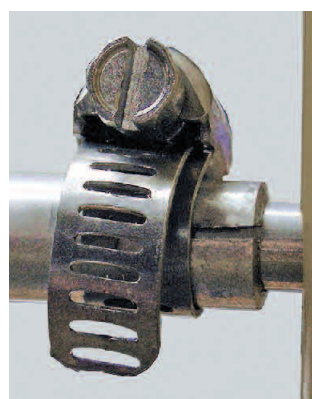
Figure 4 — An alternate method of element construction uses small hose clamps.
