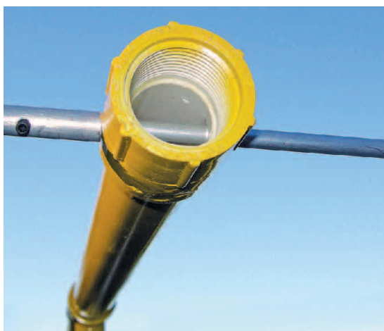
Figure 2 — Detail of reflector center. The threaded yellow piece is the end of the boom. The boom is a piece of PVC pipe (shown in yellow) which also serves as a storage case. When you take the antenna apart, all parts slide into the boom through the standard PVC to the threaded adapter, and a threaded PVC pipe cap screws into the hole to close the case/boom. The cap is removed in the photo to show the construction of the end of the antenna.
