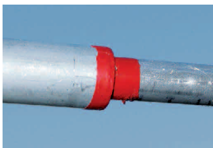
Figure 3 — Paint marks on driven element showing proper extension distance. See the text for dimensions.
