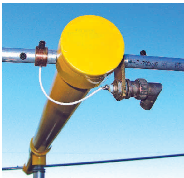
Figure 5 — Detail of feed-line connection to driven element. I did not use a current choke or a balun at the feed point.
